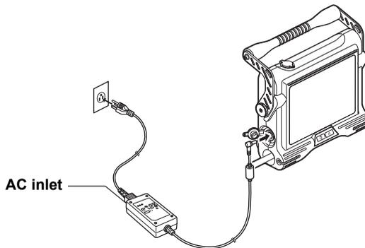
After connecting the AC power cord to the AC inlet of the AC adapter, plug the plug end of the AC power cord securely into a 3P power outlet.
