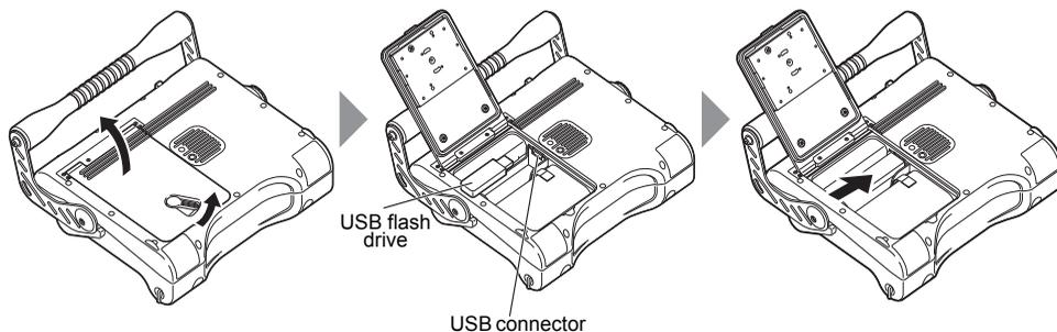
Slide the lock release lever to the side to open the battery cover.
