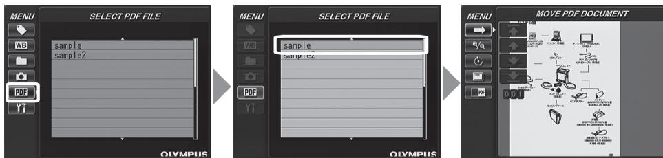
From the menu in the live screen/freeze screen, use the [BRT ▲]/[BRT ▼] buttons to move up and down and [W]/[T] buttons to move left and right to display the list of PDF files.
