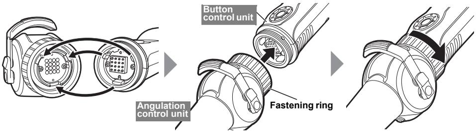
Align the notch on the angulation control unit with the protrusion on the button control unit to connect them, and firmly tighten the fastening ring in the direction of the arrow as far it can go.
