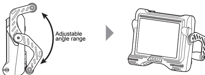
When installing the main unit on a flat surface for observation, use the handle as a stand.
