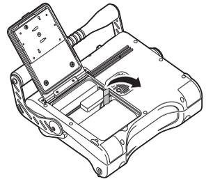
If you find it difficult to remove the battery, hook your finger directly onto the battery to remove it.
