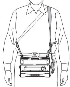
**1** Attach the shoulder belt hooks to the two belt brackets and one of the two belt holders.
