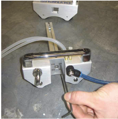
Figure 2-3 Removal of the frame screws behind the encoder assembly
