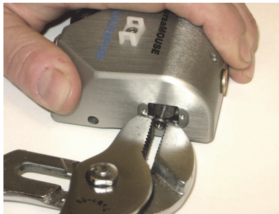
Figure 3-3 Pulling the shaft out of the VersaMOUSE
