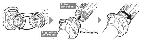
Align the notch on the angulation control unit with the protrusion on the button control unit to connect them, and firmly tighten the fastening ring in the direction of the arrow as far it can go.
