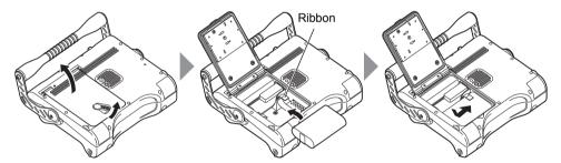
Slide the lock release lever to the side to open the battery cover.
