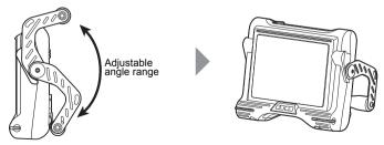
When installing the main unit on a flat surface for observation, use the handle as a stand. Adjust the handle to an angle that allows the LCD monitor to be easily viewed. The angle of the handle can be adjusted smoothly to any position within the range shown in the figure above.
