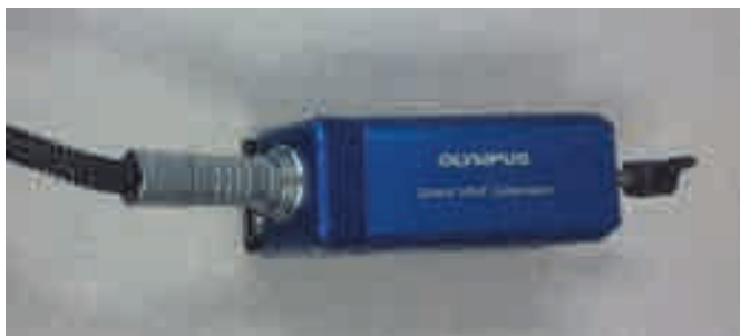
Figure 2-7 Connecting the cable to the probe
