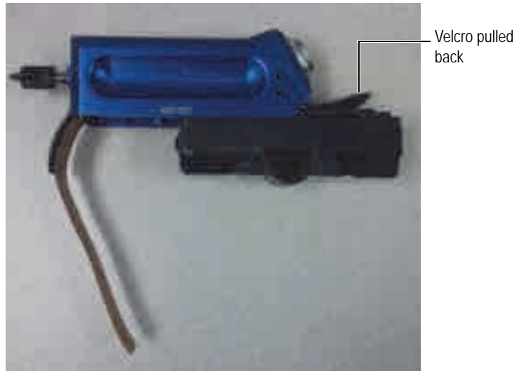
Figure 2-5 Sliding the wedge onto the probe
