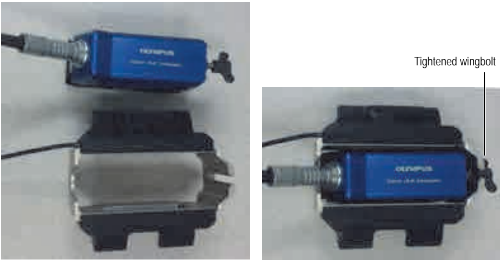
Figure 2-8 Installing the probe onto the MagnaFORM
