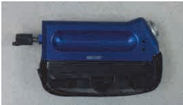
Figure 2-6 The Velcro strap wrapped around the probe and wedge
