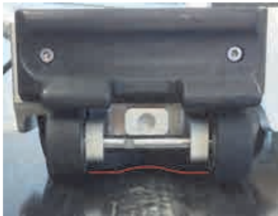
Figure 5-2 The probe's shape against the weld (red line)
