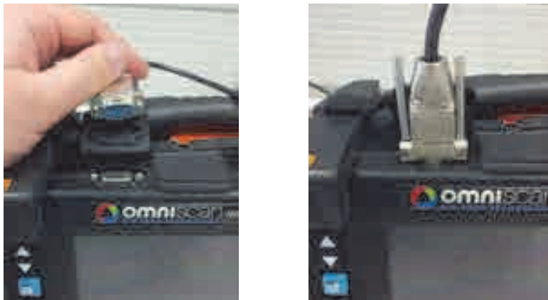
Figure 2-12 Connecting the encoder cable to the OmniScan MX
