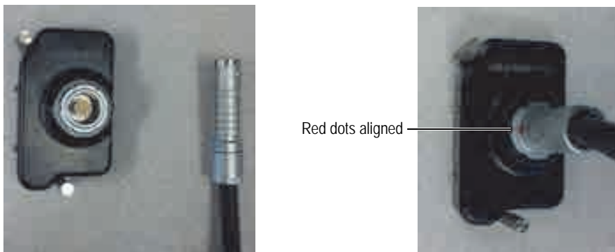
Figure 2-10 Connecting the cable to the adaptor
