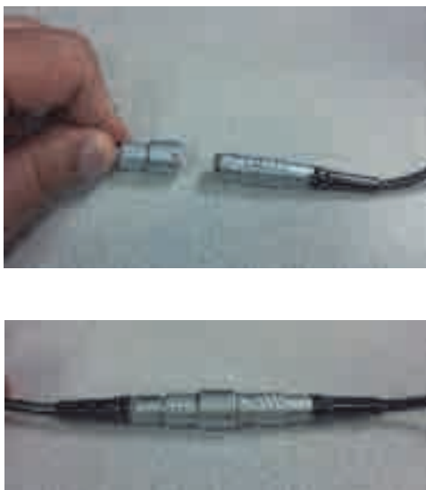
Figure 2-9 Joining the sections of the encoder cable
