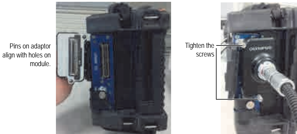
Figure 2-11 Connecting the adaptor to the OmniScan MX
