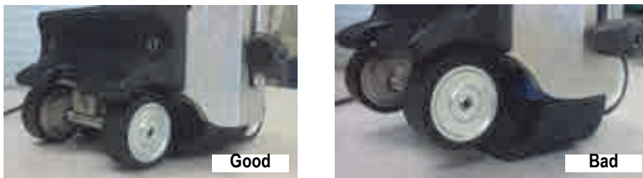
Figure 5-1 Examples of good ( left ) and bad ( right — too low) probe positions
