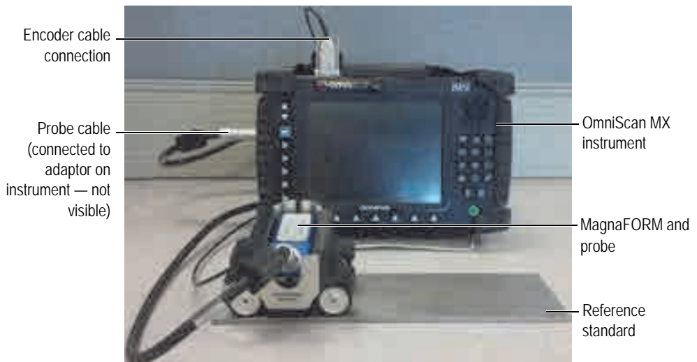
Figure 1-1 An example of an inspection setup
