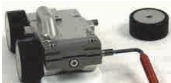
Figure 2-27 Using the supplied universal tool to install the magnetic wheels
