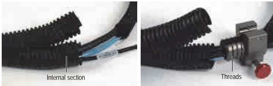
Figure 2-17 Inserting the threaded portion of the strain relief into the cable sheath
