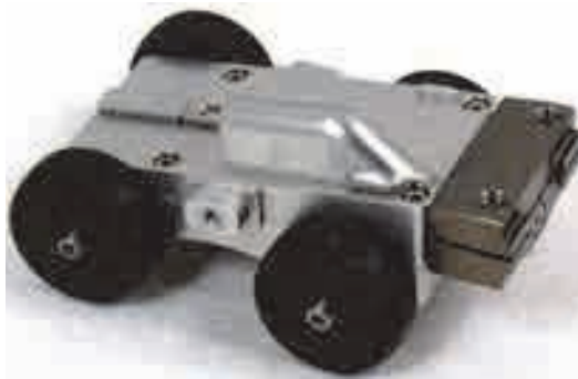
Figure 2-28 Magnetic wheels to hold the mouse scanner on ferromagnetic surface
