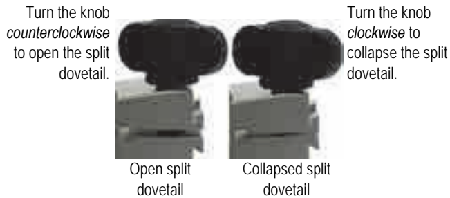
Figure 2-8 Collapsing and opening a split dovetail
