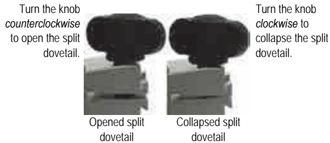
Figure 2-2 Collapsing and opening a split dovetail
