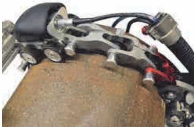
Figure 2-19 Connecting the umbilical cable to the ChainSCANNER's main module
