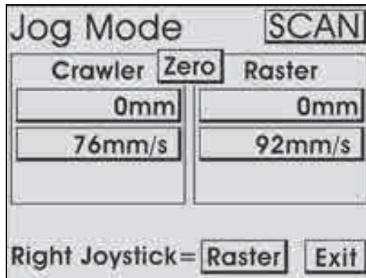
Figure 3-16 Jog mode with raster arm
