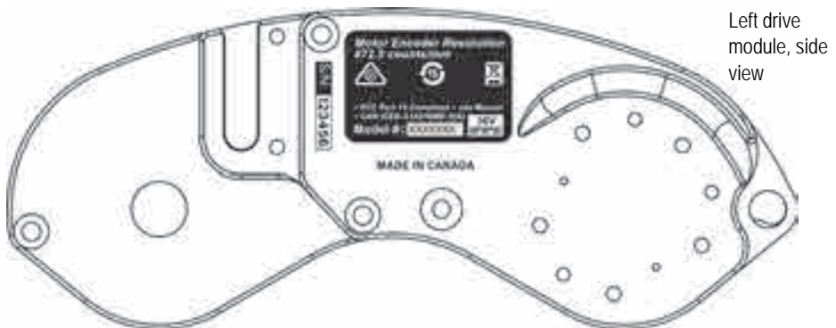
Figure i-3 Label and engraving locations on the SteerROVER left drive module
