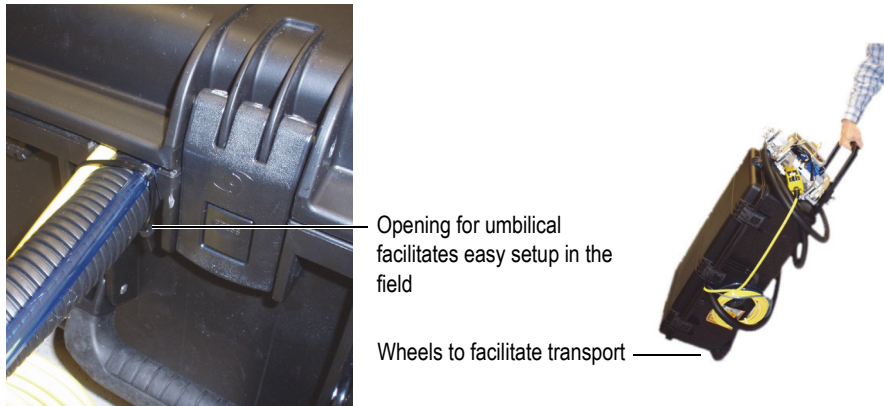
Figure 5-4 WeldROVER—transporting the system in the field
