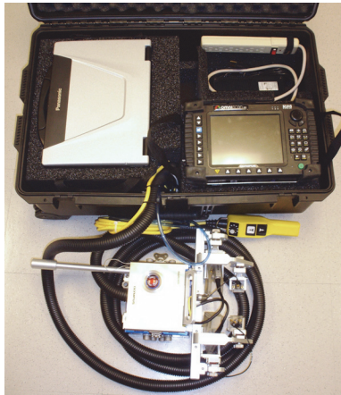
Figure 5-3 WeldROVER hard carrying case—mobile workstation configuration
