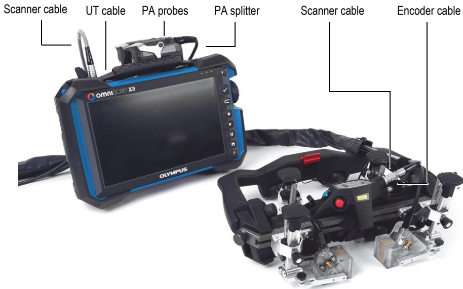
Figure 2-28 Scanner and OmniScan connected
